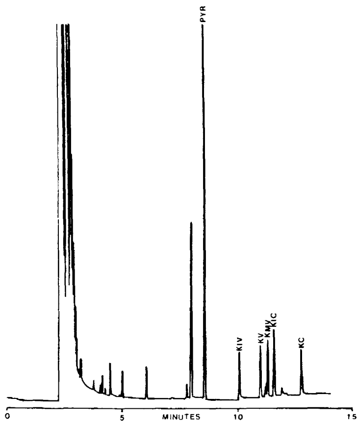
Fig. 5. Chromatogram of branched-chain \alpha -keto acids in rat whole blood. Abbreviations are defined in the text. Attenuation: 32 \cdot 10^{-12} A/mV. Chart speed: 1 cm/min. Internal standard concentration (KV and KC): 10 \mu M each.
